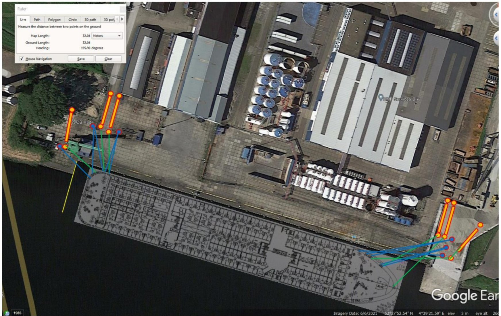
Figure 2 - Concept mooring layout. For reference, the yellow line behind the ship's stern has a length of 32m. The berth pocket has a length of 217m (corner-corner along the quay). Orange – ShoreTension and their lines, blue – ship lines.
